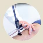
Support the stem on the leg and reset the device
